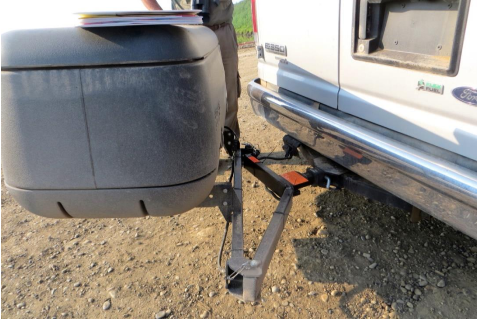
Bent I-beam supporting storage container
