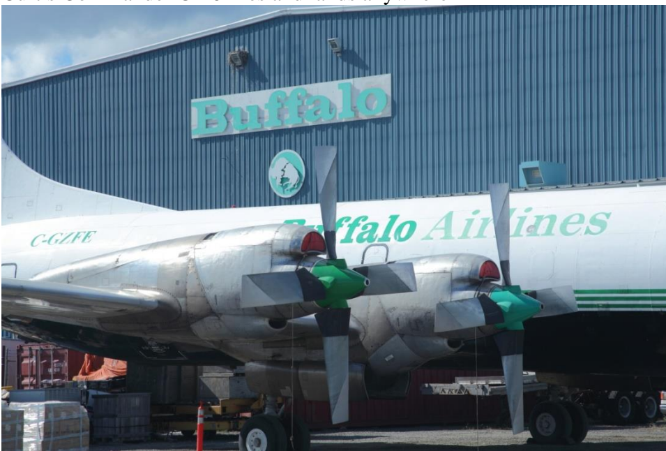
Note the square propellers on this Electra used for far north flights
