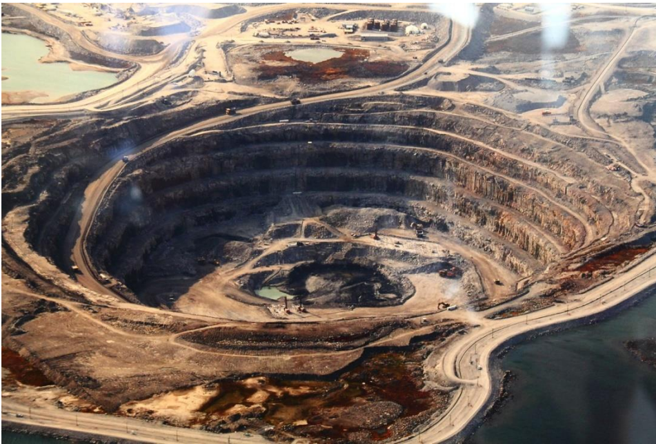
Diamond mine in summer, showing roadway spirally downward
